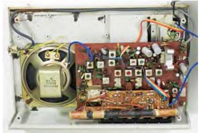
View inside the Model 56 multiband receiver with back cover removed. (Picture is rotated 180° to match sketch below.)
