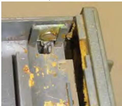
The battery compartment showed signs of corrosion at the positive connector.
