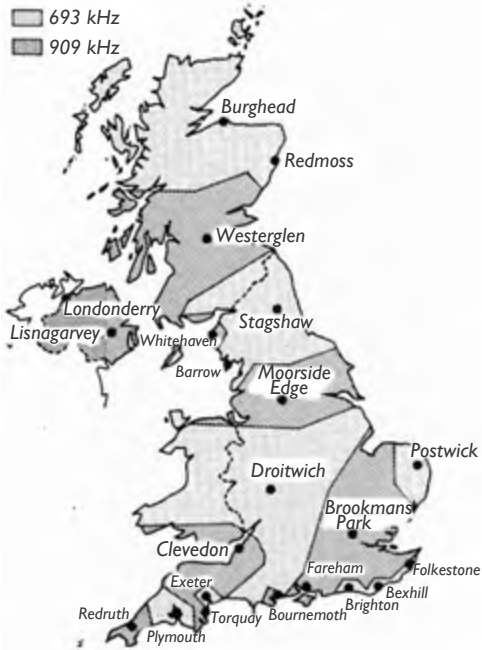
Plan for moving BBC Radio 2 from long wave to two medium frequencies, 693 and 909 kHz.
