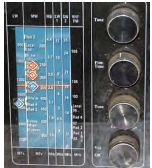
Analog tuning dial of WHSmith Model 56 receiver was marked with positions of BBC stations “Rad 1” to “Rad 4”.
