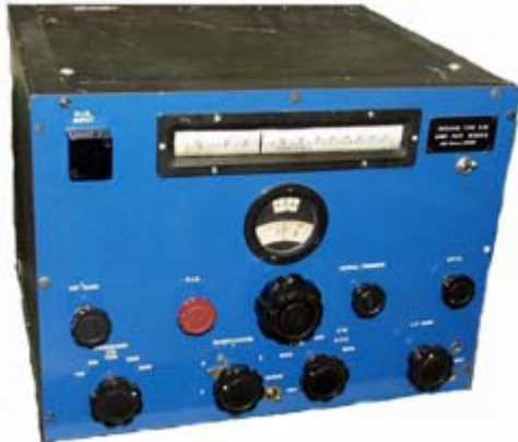
World War II B28 communications receiver was the British Admiralty's version of the Marconi CR100.
