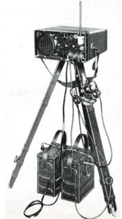
British Army B44 AM transceiver for 60-95 MHz AM, mounted on tripod with batteries below.
