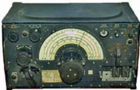
Marconi R1155L MF/HF receiver as installed in Avro Lancaster bombers, with a companion T1154 transmitter.
