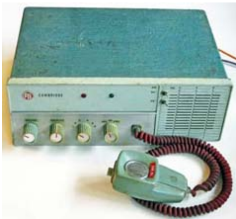
Pye Cambridge mobile radiotelephone with all solid-state receiver and transistor inverter for the vacuum tube transmitter.
