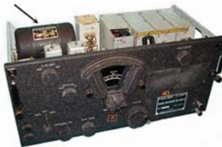
BC-348 HF receiver as used in USAAF aircraft of WWII. Internal dynamotor (arrowed) provided +220V DC.
