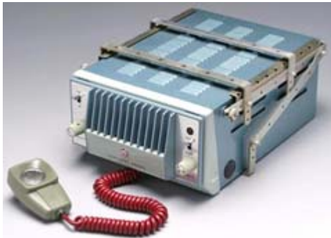
Pye Transistor Ranger radiotelephone with front panel heat sink for inverter transistors. [Credit: Science Museum CC BY-NC-SA 4.0.]
