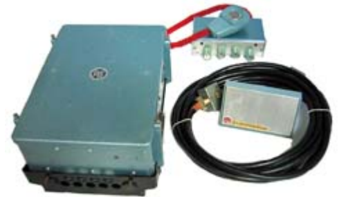
Trunk-mount Pye Cambridge with remote-control box, microphone, loud-speaker and connecting cable.
