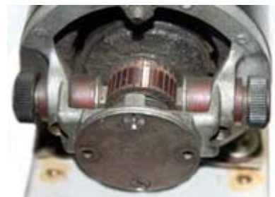
Commutator and brushes of a BC-348 receiver's dynamotor. There is another commutator at the far end of the dynamotor.
