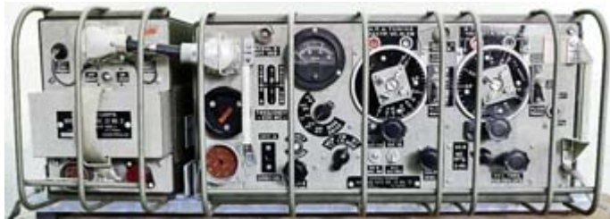
Wireless Set No. 19 as employed in WWII tanks and Jeeps. Dynamotor power supply at left. [CC BY-SA 4.0, Autopilot]
