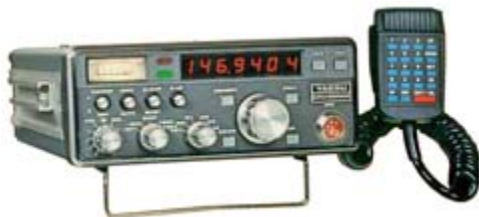
Yaesu CPU-2500R transceiver from 1979 covered 144-148 MHz with four memory channels, scanning and 25W power out.
