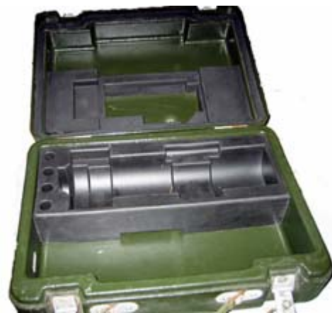
Original interior of the military case, with rubber moldings designed to hold a KITE image-intensified night sight. [KD2EVI pic.]
