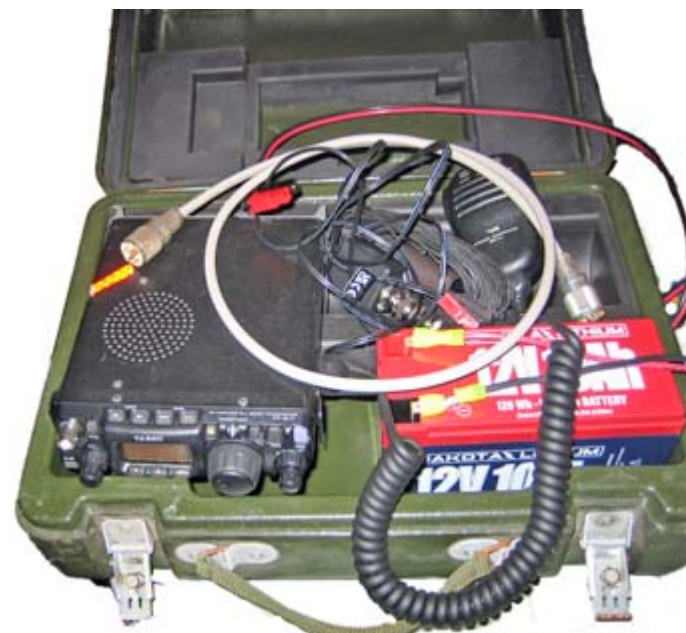
Military case holding Yaesu FT-817 multimode QRP transceiver covering 160-10m, 6m, 2m and 70cm bands, 10Ah LiFePO 4 battery, antenna and feeder. [KD2EVI pic.]
