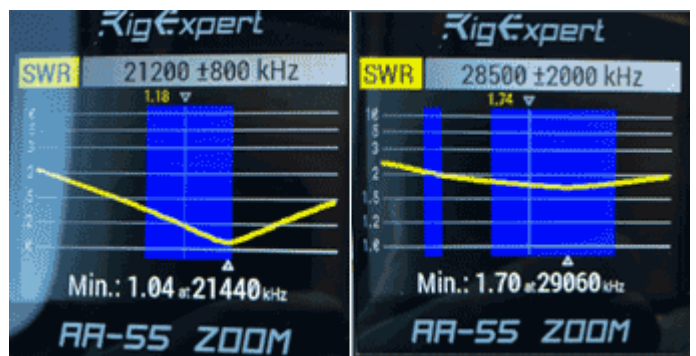
SWR plots of HD-330 screwdriver antenna on 15 meters and 10 meters.
