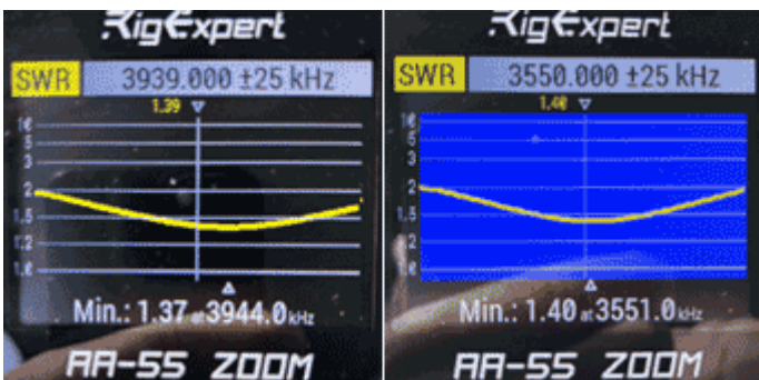
SWR plots for 75 meters and 80 meters using RigExpert AA-55 ZOOM antenna analyzer. [K2WPM pics.]
