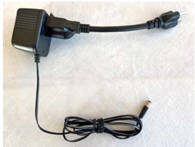
A short electrical extension cord allows a low voltage power supply to be used with a crowded power strip. [N2KZ pic.]
