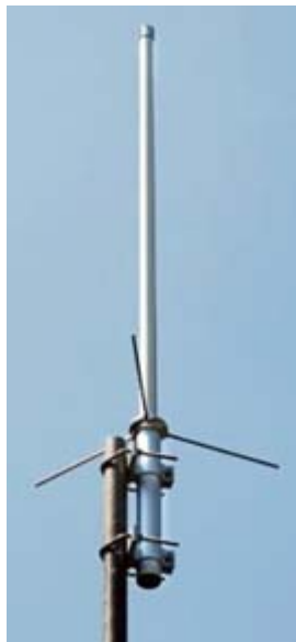
Comet GP-1 antenna is just 4.2 ft high, covering 144-148 MHz and 442-450 MHz.
