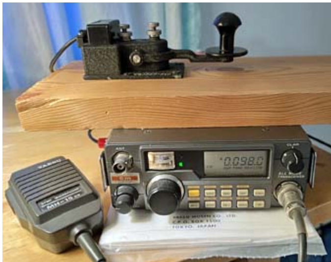
Yaesu FT-690R II transceiver covers 50 - 54 MHz with 2½ watts output barefoot. [N2KZ pic.]
