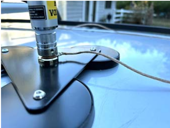
Close-up of magnetic mount on vehicle roof with counterpoise wire slipped over the SO-239 connector.
