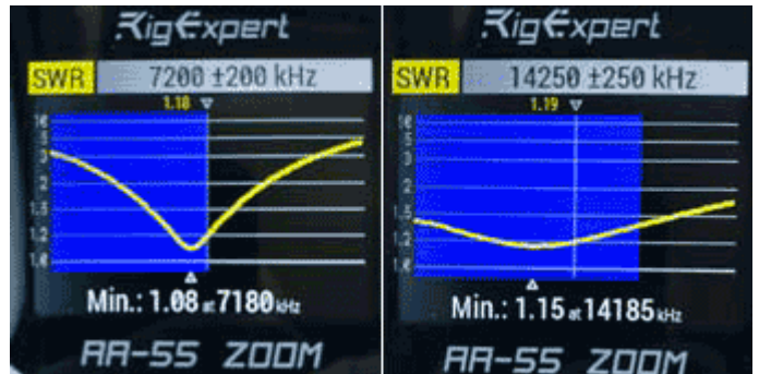
SWR plots of HD-330 antenna on 40 meters and 20 meters.
