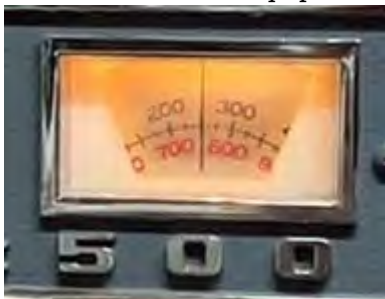
Sommerkamp FL-500 transmitter's analog VFO dial.
