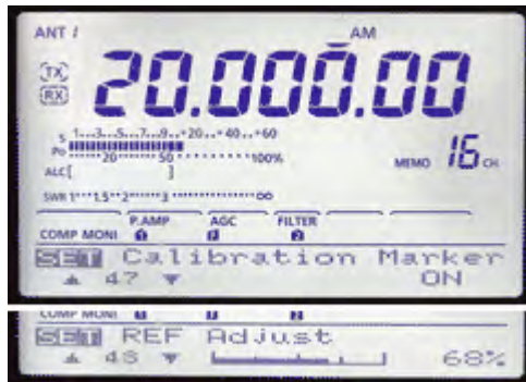
Icom IC-7410 can turn on a calibration marker with Set Menu item #47 (top). Adjustment of reference oscillator is available with Set Menu item #48 (below).
