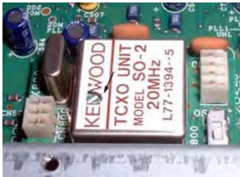
Adjustment point (arrowed) for the reference oscillator in the SO-2 TCXO unit of a Kenwood TS-870 HF transceiver.
