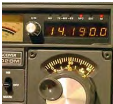
Yaesu FT-902DM transceiver from 1981 had a free-running VFO with built-in digital frequency counter.
