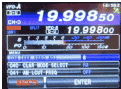
When using WSJT-X in FreqCal mode, tcvr frequency jumps from 20.000 to 19.9985 MHz
