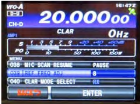
Adjustment of Reference Frequency through menu item 039 of the FT-991A.
