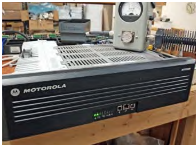
New Motorola MTR3000 repeater producing 50 watts output while on-test into dummy load. [N2CBH pic.]
