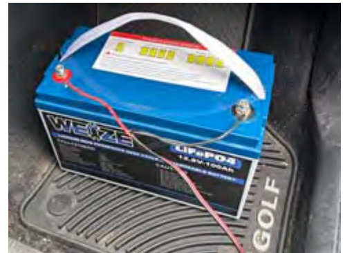
Weize 12.8V 100Ah LiFePO 4 battery weighs 2.6 lbs and is less expensive than Bioenno. [K2WPM pic.]
