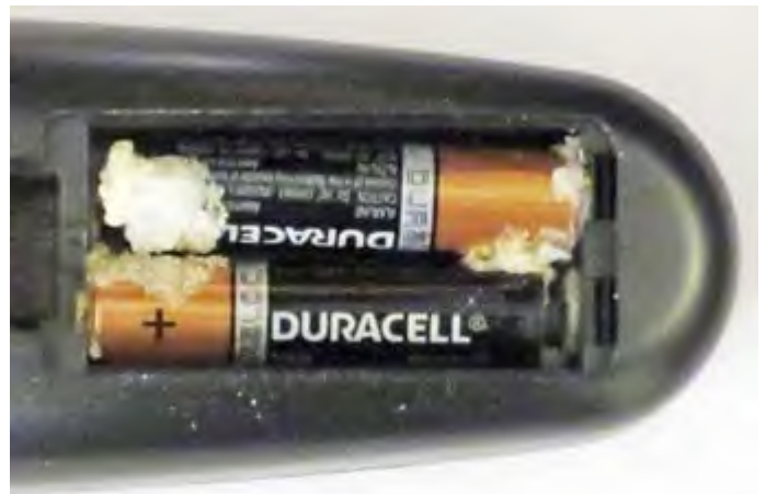
Two AAA alkaline cells left inside a remote control that was not used for over a year.
