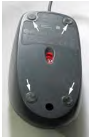
Clean the sliding pads (arrowed) underneath your computer mouse.
