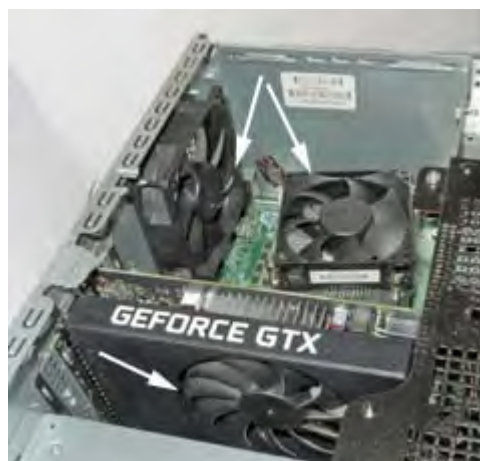
This desktop computer has a chassis fan, a CPU fan and a third fan built-in to the graphics adapter, all arrowed. A fourth fan is inside the power supply.
