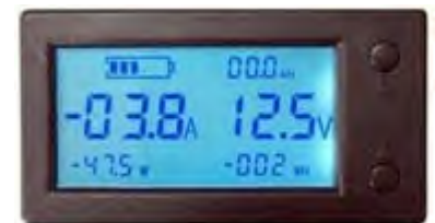
DYKB battery monitor has a Hall effect sensor for contactless current measurement.
