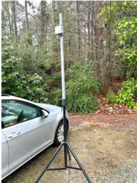
49:1 balun with EFHW wire attached, mounted on PVC tube and Pyle speaker tripod. [K2WPM pic.]
