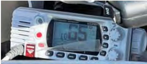
Standard Horizon Eclipse marine VHF FM radio is waterproof with DSC (digital selective calling) capabilities. [N2KZ pic.]
