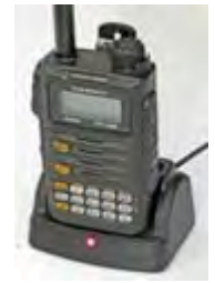
HT with drop-in charger. Yaesu FT-70 has a lithium-ion battery.
