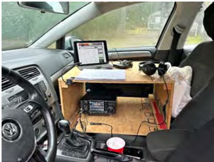
K2WPM mobile cabinet on the passenger seat houses the Icom IC-7300, iPad, log and CW key. [K2WPM pic.]
