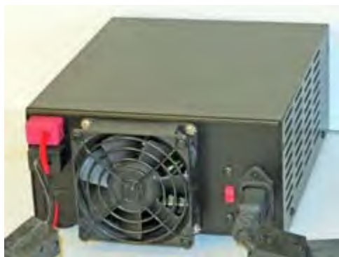
Large cooling fan on back of SS-30M power supply after cleaning. Unusually, this fan draws cool air into the chassis.
