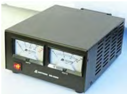
Astron SS-30M switch-mode 12 volt 30 amp power supply. [Pics - NM9J]
