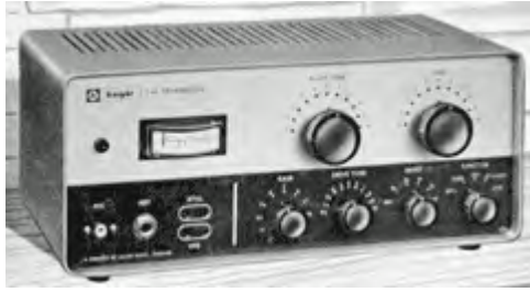
Knight T-60 was a kit-built AM and CW transmitter covering 80 - 6 meters, running 60 watts to a 6DQ6 vacuum tube.
