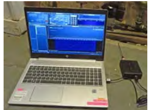
Monitoring emissions from the new ProCoder)R900i water meter using SDR-Play's RSP1A wideband SDR receiver connected to a Windows notebook computer.
