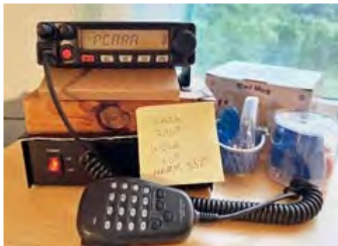
Yaesu FT-1900 is capable of 55 watts output on 2 meters.
