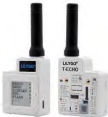
Lilygo T-Echo with LoRa, Bluetooth, antenna and E-paper display.
