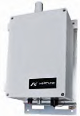
Gateway fixed network data collector is mounted on a high spot and connected to an external 911 MHz antenna. Cell network antenna is on top.
