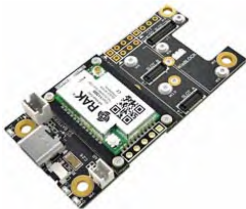
RAK WisBlock base board with LoRa wireless module plugged in.
