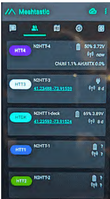
The Meshtastic app displays a list of nodes that have been heard. [N2HTT pic.]
