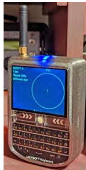
Lilygo T-Deck housed in a 3D-printed case by Mike N2HTT. [N2HTT pic.]
