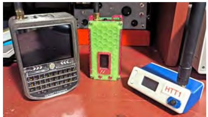
A variety of 3D-printed enclosures for LoRa devices used in Meshtastic. [N2HTT pic.]
