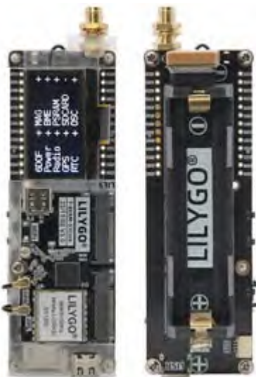
Lilygo® T-Beam LoRa wireless module with OLED display and battery connector also supports an optional GPS module.
