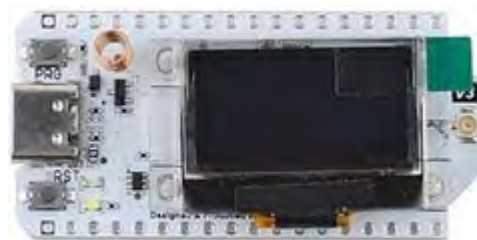
Heltec WiFi LoRa 32 V3 Internet-of-Things development board based on ESP32-S3 microcontroller, has USB type C, Wi-Fi, Bluetooth Low Energy, LoRa and an OLED display.
