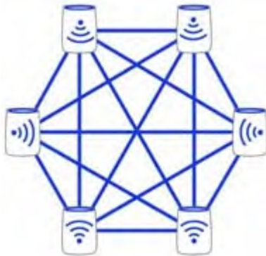
Wireless mesh network. Each node can pass a message to another node that is in-range.
