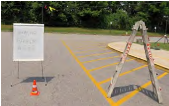
Whiteboard, safety cone, step-ladder and hazard tape mark the presence of low-hanging feeder for the dipole.
