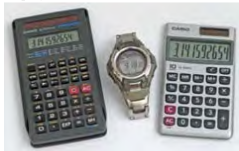
Two Casio calculators and “Tough Solar” wrist watch powered by solar cells.
