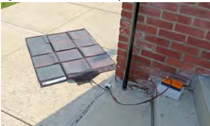
Mike W2IG's fold-out solar panel charges the 12V lithium battery (at right).
