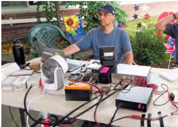
Lou KD2ITZ makes “Alternate Power” contacts with the FT-450D connected to a solar-charged lithium battery.
