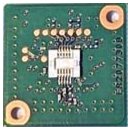
Yaesu SPU-1 audio signal processor can be installed in the FT-3165, FT-3185, FTM-150, FTM-510.
