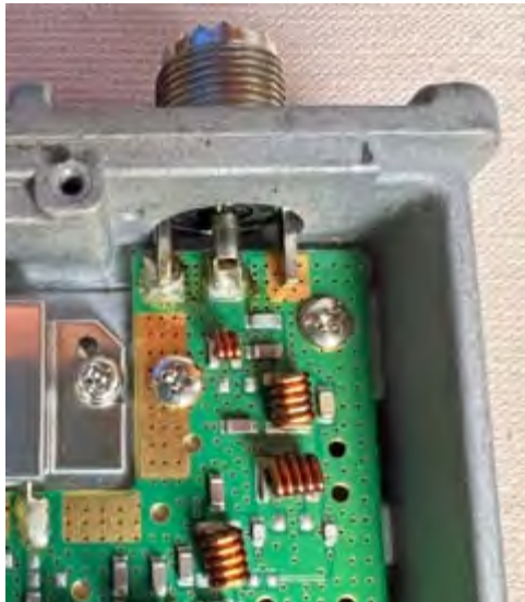
FT-1900 antenna connector was soldered to the circuit board. [N2KZ pic.]
