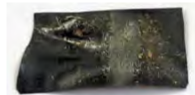
Vinyl tape removed from antenna was contaminated with sand.
