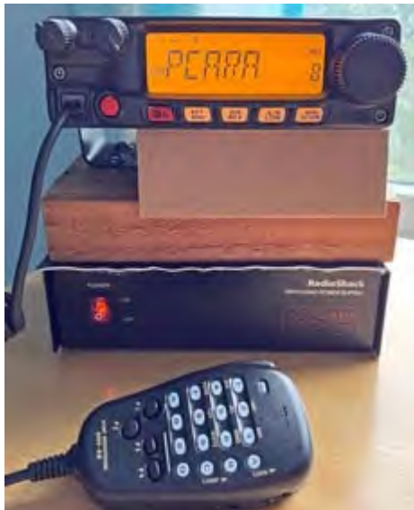
The FT-2980 memory channels can be displayed with channel frequency or a 6-character alpha-numeric label. [N2KZ pic.]
