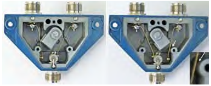
MFJ-1702C two-position coaxial switch. As cam rotates, it grounds the unused port and allows springy contact of connected port to touch the common connector. A worn switch can be parked with the unused port not fully grounded (inset arrow). [NM9J pic.]
