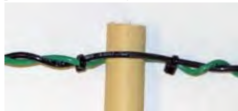
Black nylon cable ties keep the antenna wires in place on the plastic spacers.
