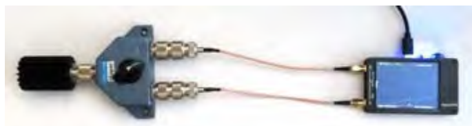
NanoVNA (right) is connected to an MFJ-1702C 2-position coax switch to measure the leakage from port A to port B.
