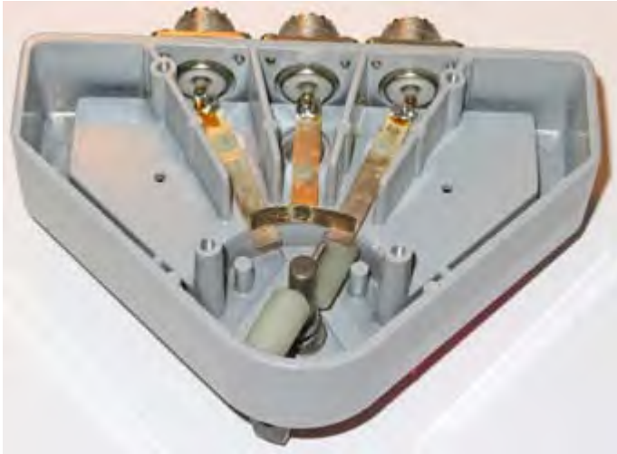
Alpha Delta DELTA-2 coaxial switch with cover removed. As knob is turned, plastic cylinder raises end of metal strip (right) from chassis ground so it connects to the common port's curved metal strip. [NM9J pic.]
