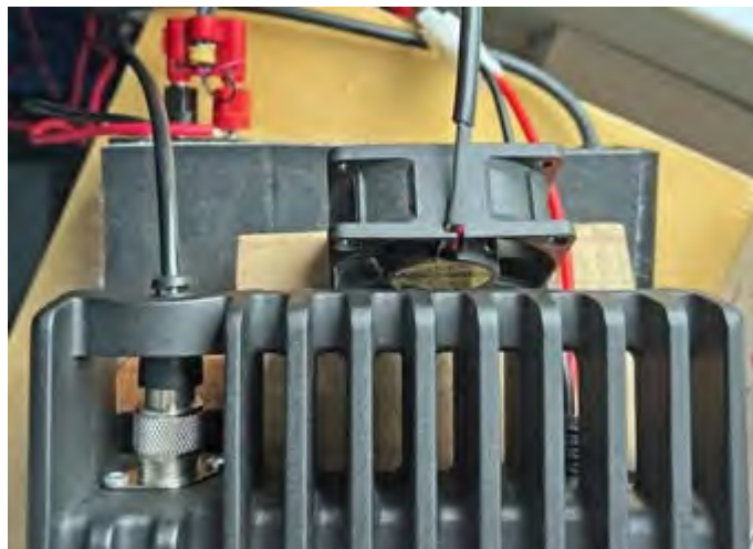
A small muffin fan was added to force air across the substantial heat sink. [N2KZ pic.]
