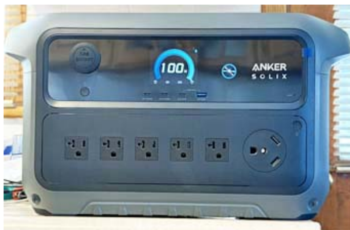
Anker Solix C2000 Gen 2 Portable Power Station has 2,048 watt-hours of capacity, providing up to 2,400 watts of AC power from internal LiFePO 4 batteries. [KD2EVI pic.]
