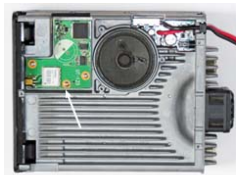
UT-123 Digital/GPS Unit (arrowed) mounted under the top cover of the Icom IC-2820H transceiver.
