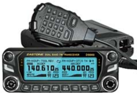
Zastone D9000 dual band FM transceiver transmits on 136-174 MHz and 400-480 MHz with 50 watts (VHF) and 40 watts (UHF).
