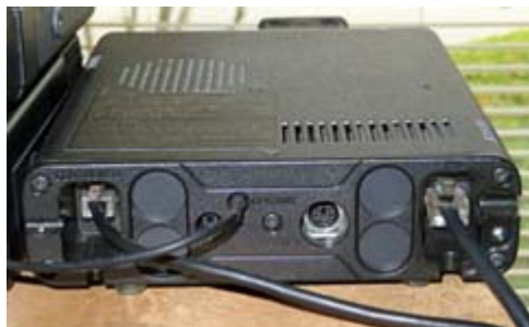
IC-2820H main unit on top shelf. Separation cable from controller is plugged into the left-hand jack, microphone is plugged into right-hand jack.
