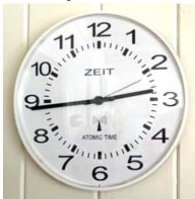
"Atomic" clocks decode bits from WWVB on 60 kHz to indicate when DST is in effect.
