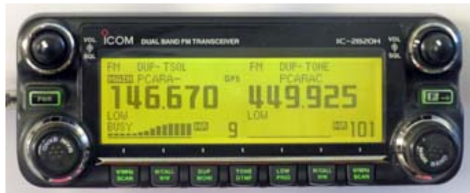
Icom IC-2820H transceiver front panel. Seven-segment S-meter indicates a strong signal on 146.670 MHz.
