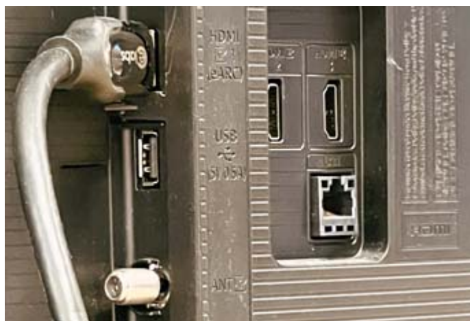
HDMI cable (left) connected to HDMI 1/eARC connector on a modern Samsung TV. The other connectors are for HDMI 2 and HDMI 3, USB, F-coaxial antenna and Ethernet local area network. [N2KZ pic.]
