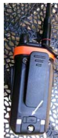
Location of USB-C charging port (arrowed) on rear of UV-21R battery. [KD2EVI pic.]
