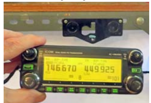
Magnetic mounting of control head (amber backlight) to remote controller bracket.
