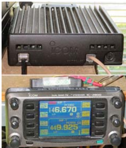
Old Icom IC-2800H dual band transceiver with separate control head and backlit color display. A pair of fans kept the control head cool in summer.
