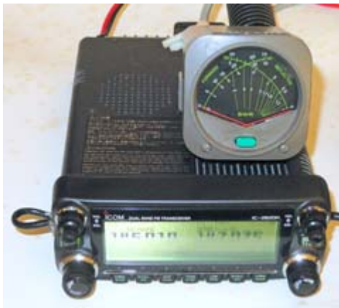
IC-2820H transceiver with control head mounted on the main body for initial testing. Power meter and dummy load were connected to the [ANT1] SO-239.
