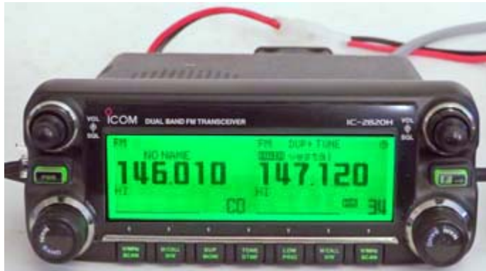
IC-2820H with dot-matrix display backlight set to original green. Front panel buttons are also backlit green.
