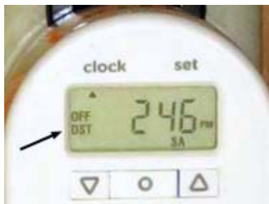
Electrical timers may have a DST option (arrow).
