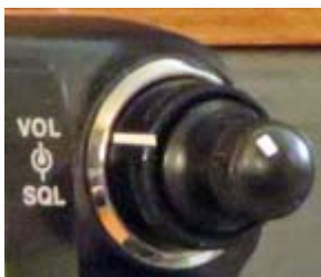
Right hand VOLUME/SQUELCH control knob with white vinyl strips.
