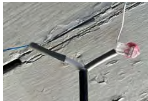
Center of Karl's improvised FM dipole with Scotchlok splice on the right.
