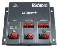
West Mountain Radio ISOpwr+ isolates and charges a 12 volt auxiliary battery.
