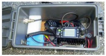
Go-box described by David KD2EVI in PCARA Update, September 2023. Lower left: 4.5 Ah LiFePO4 battery with AC charger. Lower right: TYT TH-8600 VHF/UHF transceiver inside the ammo box. [KD2EVI pic.]
