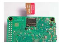
Inserting a 64GB microSD card into the Raspberry Pi 5.
