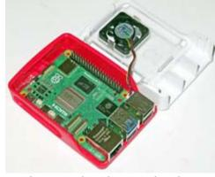
Raspberry Pi 5 board mounted in the official case. White frame contains the case fan, which is wired to the board.
