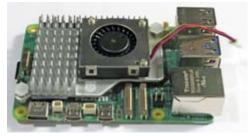
Raspberry Pi 5 Active Cooler mounts onto the RPi 5 board with two push-pins.
