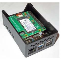
HighPi Pro 5S plastic case with Raspberry Pi 5 and solid state drive mounted inside. The ventilated case lid, which clips on top, is not shown.
