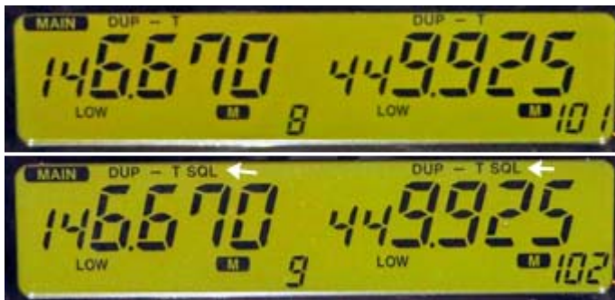
Top: display on Icom IC-2720 FM transceiver shows two memories with CTCSS tone on transmit (T). Below: adjacent memories with tone squelch (T SQL), arrowed.
