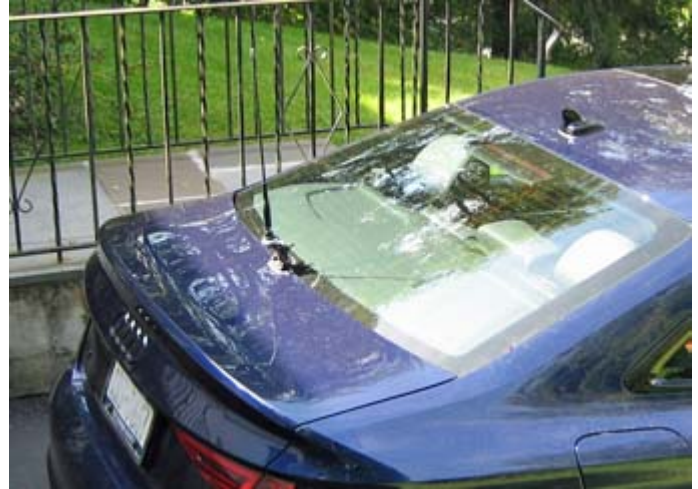
Comet CP-5 adjustable lip mount and Comet SBB-1 16" dual-band antenna. [KD2EVI pic.]
