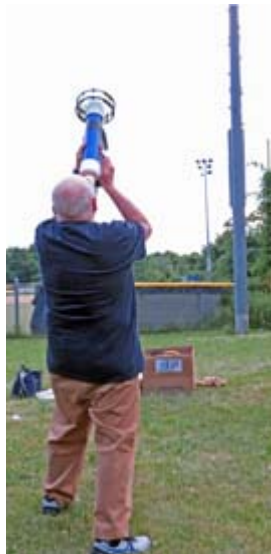
Charles N2SO uses his CSV17 launcher to send lines over light poles at Field Day.
