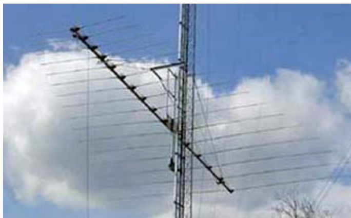
Telrex 143042-105 16-element log periodic antenna covers frequency range of 14 - 30 MHz with a 42 foot boom. (If you need to ask the price, you can't afford it.)
