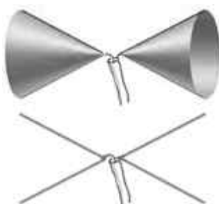
Wideband biconical dipole simplified to 'X' antenna.
