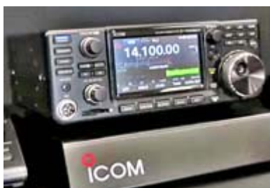
Icom IC-7300Mk 2 transceiver now has an HDMI external display connector, SMA RX in/out connectors, CW decoder, USB-C and Ethernet ports.
