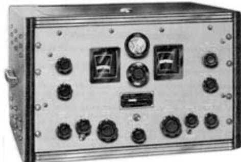
Hammarlund SP200 receiver covered 0.1 to 40 MHz in five frequency bands.
